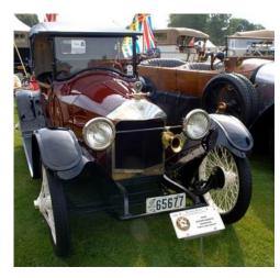
**A19:** The 1915 Scripps-Booth Model C. The car also was the first with electric door latches.
